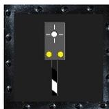
The board "Ne5" on the platforms indicates where the front of the train should stop in order to enable optimal boarding.
