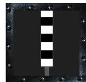
The signal "So16" uses a white flashing light to indicate that the associated level crossing is secured and the train can approach to it.
