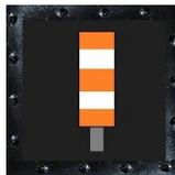
The light signal "So18" indicates an automatic switch and its position. In addition to a control light, a second light indicates, the switch is in default position.
