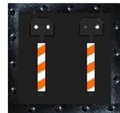
Signals of the type "Wn" indicate a switch and the chosen track beyond that switch.
