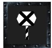
The trapezoidal sign "Ne2" serves as an entry signal on routes without electrical signals; for example on the "Selketalbahn". Without permission to proceed into the station, you have to wait for further instructions there.
