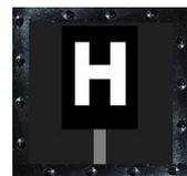
The sign "Sh0" marks the end of track. It can be found on the buffer stops, for example, and indicates that the track is impassable from here always.
