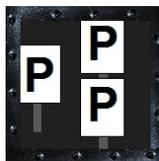
The signal So15 announces the monitoring signal So16 for secured level crossings (BÜ). The electric contact is at this point.
