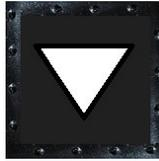
The signal "Ne2" announces a main signal. The speed must be adjusted so that a stop would be possible.
